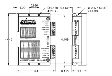
If you're looking for big time stepper performance from a small driver, the MBC061281 is your answer. This powerful microstepping driver provides excellent torque in a compact and low profile enclosure. The MBC061281 is also very easy to use. It features rugged terminal blocks, a dip switch for current settings, and a visible silkscreen for easy installation and configuration.
